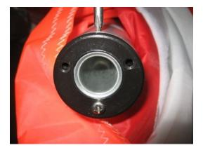
• Using a pair of needle-nose pliers pushed into the two holes in the head of the cam, rotate the cam to the degree desired. In the example described above, the cam will have to be rotated 5 mm clockwise.
